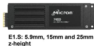
**How to use:** 15mm z-height enables greater power and heat dissipation while 7mm z-height means more SSDs can fit into the same chassis. The Micron 7400 SSD is uniquely offered in an optional 15mm form factor and E1.S. The standard E1.S form factor is commonly used in ultradense storage server and storage platforms.
